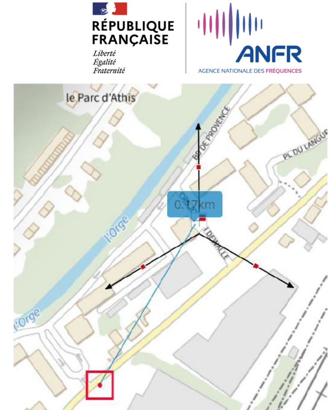
Measurements in 3400-3490 MHz : SFR base station located at 170 m from the receiver (red square), with a clear line of sight
